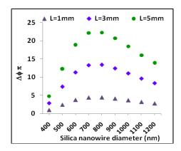
Figure 1: Phase difference in the two arms of Mach-Zehnder interferometer
